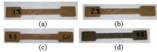
Fig. 4. Specimens for the composition of variations in table 1: (a) V1.1, (b) V1.2, (c) V1.3, and (d) V1.4
