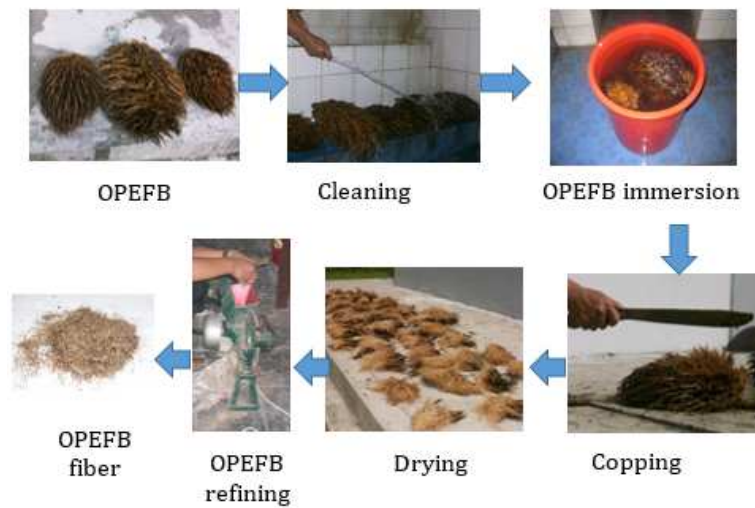
Fig. 1. Process for preparing OPEFB fibers
